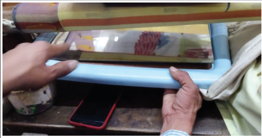
Figure 2. The Kota Fabric is Woven Upside Down and the Front Design can be Seen Here with the Help of a Mirror.
